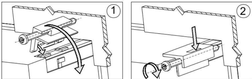
*Fig. 1. Controller fixing in the panel.*
