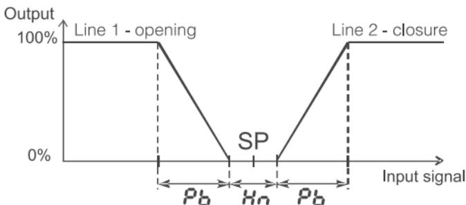
*Fig. 11. Step-by-step three-state control*
