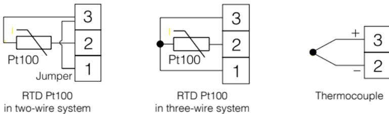
Fig. 4. Connection of input signals
