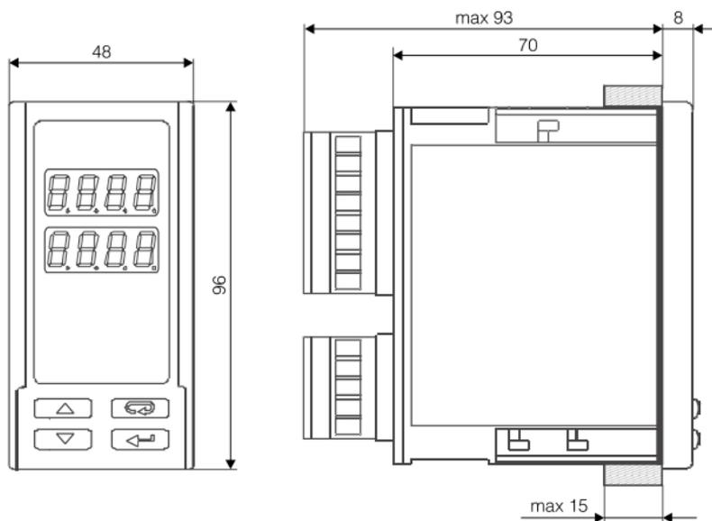
*Fig. 2. Controller overall dimensions*
