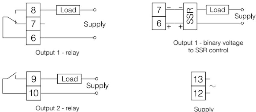
Fig. 5. Supply and load circuit connection
