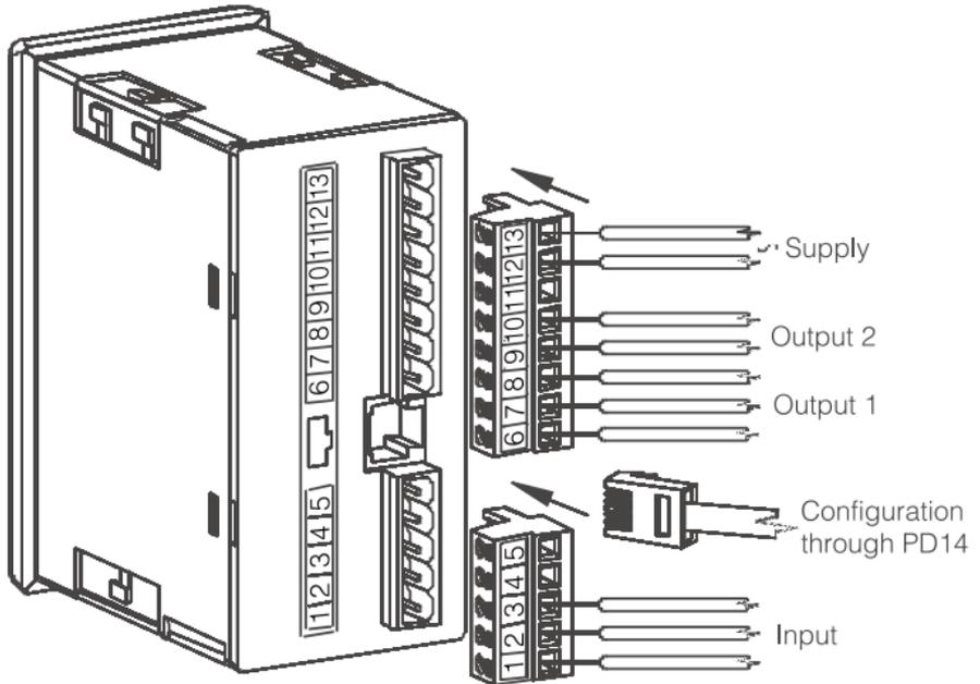
Fig. 3. View of controller connection strips
